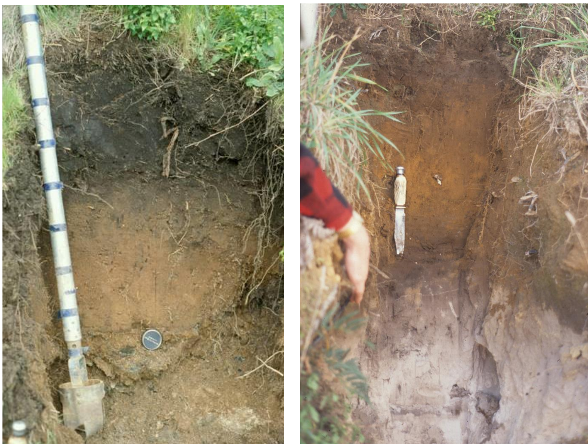
Fig. 6 (left). Profile of soil (Humic Vitrixerand) mainly on basaltic ash at Brownes Lake near Mt Gambier, South Australia (marks on auger at 10-cm intervals) (from Churchman et al., 2016c, p. 400). Fig. 7 (right). Profile of soil (Thaptic Haploxerand) on basaltic ash over a buried soil on aeolian sand at Laslett Road near Mt Schank, South Australia (knife ~25 cm long) (from Churchman et al., 2016c, p. 400)
