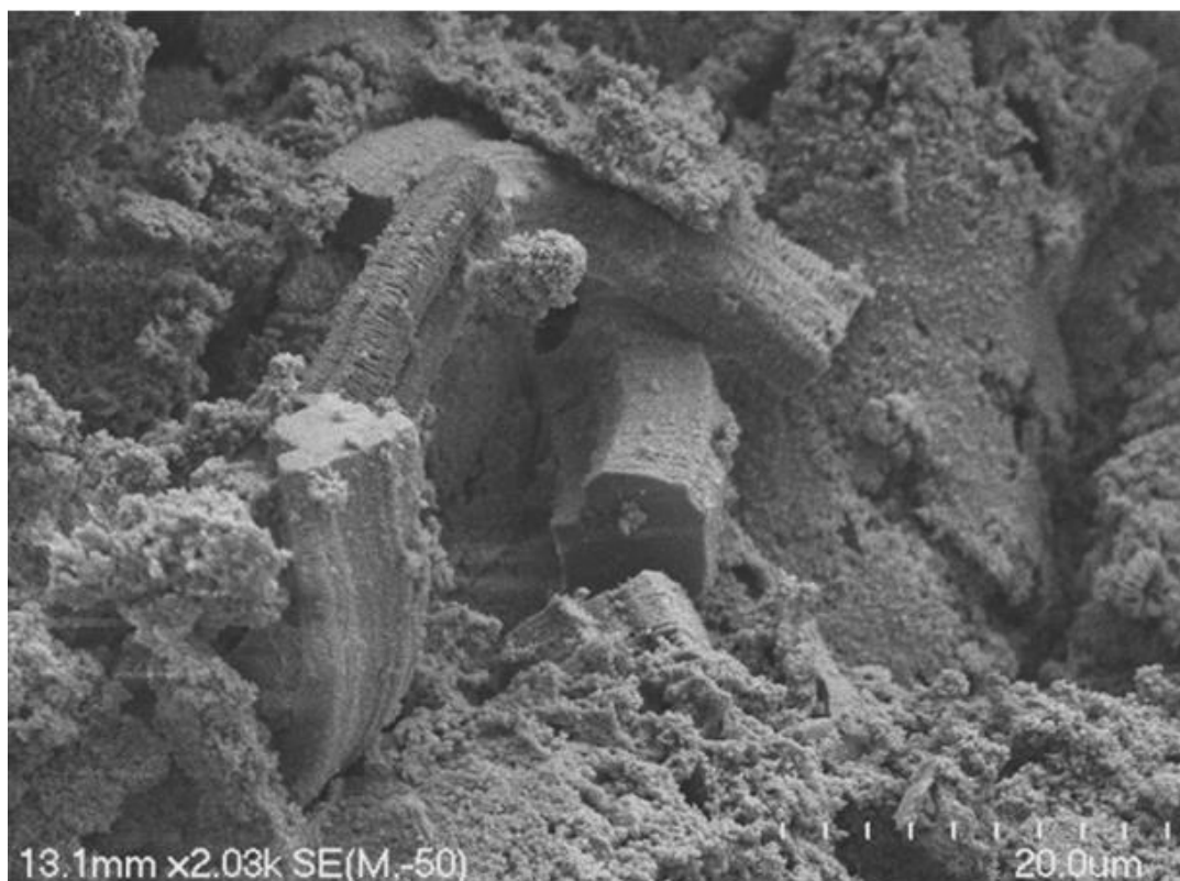
Fig. 1. SEM image showing multiple curved (vermicular) halloysite books of differing sizes in ~270,000 year-old Te Ranga tephra (Tauriko site, Tauranga). From Cunningham et al. (2016, p. 360).
